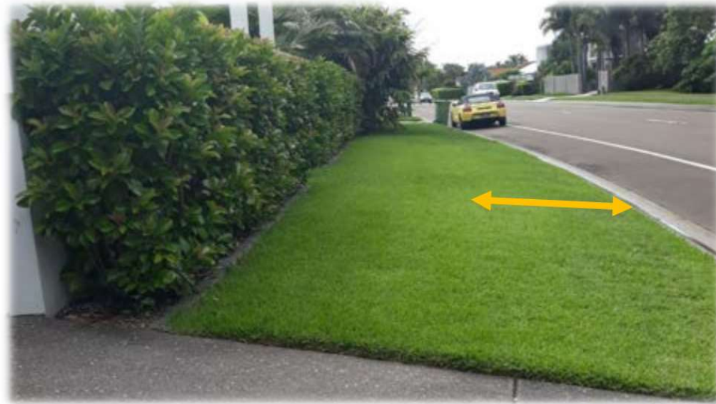
Figure 1: 1500mm minimum clearance for road functions
